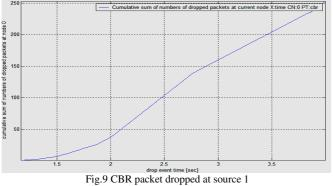
Fig.9 shows, drop of packets starts when the receiver nodes leave one multicasting group and join other. During this process prune and graft packets are generated by intermediate and leaf routers of the network. The queue starts getting full and the dropping increases. The graph shows that increase in drop of packets is below 50 before 2.05s whereas drop of packets increases 50 at 1.75s in Drop Tail queuing implementation. Total number of dropped packets is in the range of 250.
