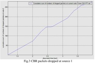
Fig.3 shows, dropping of packets starts when the receiver nodes leave one multicasting group and join other. During this process prune and graft packets are generated by intermediate and leaf routers of the network. The queue starts getting full and the dropping increases. The graph shows the increase in dropping of packets at 2.4s due to the increase in traffic since source 2 also starts sending and nodes start joining this group while leaving other.
