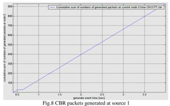
Fig.8 depicts, source 1 starts generating CBR packets after 0.4s of the start of simulation. Since the packet size is 210bytes and it is the beginning of the generation process, hence queue is empty and the graph shows the constant generation of packets in the range of 950 packets.
