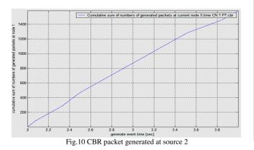
Ashish Kumar et al, / (IJCSIT) International Journal of Computer Science and Information Technologies, Vol. 3 (2), 2012,3816 - 3820 Fig.10 shows, source 2 starts generating CBR packets after 2s of the start of simulation. Number of packets generated is in the range of 1500 by the end of the simulation.
