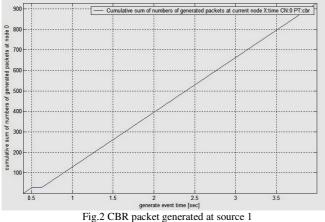
Fig.2 depicts, source 1 starts generating CBR packets after 0.4s of the start of simulation. Since the packet size is 210bytes and it is the beginning of the generation process, hence queue is empty and the graph shows the constant generation of packets in the range of 950 packets.
