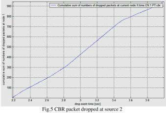
Fig.5 shows, drop of CBR packets at source 2. Drop of packets starts at 2.2s of simulation. Source 2 is the gateway of source 1, so the queue of source 2 gets full early and starts dropping of packets after 0.2s of its packet generation which is in the range of 950.
