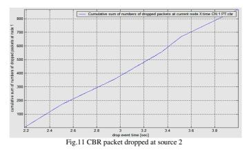
Fig.11 shows, drop of CBR packets at source 2. Drop of packet starts at 2.2s after simulation starts. Source 2 is the gateway of source 1, so the queue of source 2 gets full early and starts dropping of packets after 0.2s of its packet generation which is in the range of 800.
